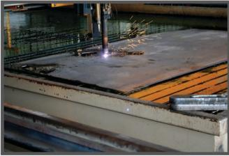
Our two CNC Plasma Cutters allow for precision and accuracy. We have complete machine shop dedicated to your crusher rebuild, replacement, and repair needs. We have boring mills up to 12 feet, lathes up to 52 inches by 25 feet, and milling machines up to 10.5 feet.
